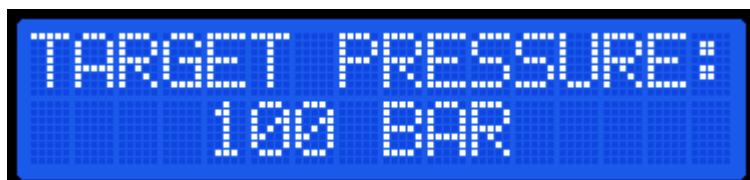
With the target pressure display visible, press the rotary control knob once to enable selection mode. A selection arrow will appear next to the pressure value. With the selection arrow visible, rotate the rotary control knob clockwise or anti-clockwise to increase or decrease the target pressure setting.
