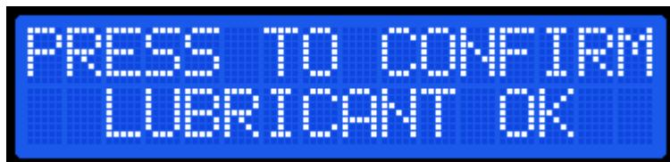
Press the rotary control knob to confirm the lubricant check. After this, the display will show the first page of the main menu; the target pressure display.
