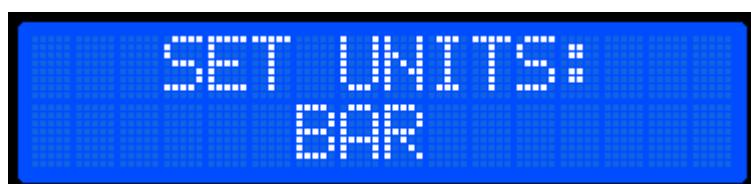
Press the rotary control knob a second time to enable selection mode. A selection arrow will appear next to the currently selected unit of pressure.
