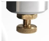
Depressurise the compressor by unscrewing the bleed screw; using a rag for this is advised. Whilst depressurising, some moisture and silicone may be expelled from the water separator. Suitable precautions should be taken to protect any floor coverings under the compressor.
