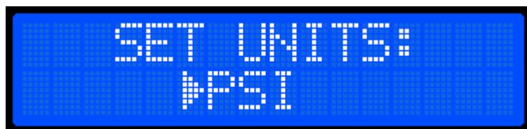
Rotate the rotary control knob in either direction to cycle between the selectable units. Once the desired unit is visible, press the rotary control knob once to save the selection. The compressor will retain the selected pressure unit, even after being powered off.
