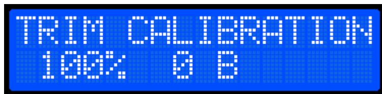
The default settings for trim calibration are 100% scale and 0 BAR offset. It is NOT advised that users change these settings without having observed a consistent inaccuracy in indicated pressure.
