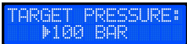
Once the desired target pressure is displayed, press the rotary control knob once to confirm the target pressure selection. After confirming the target pressure selection, the start display at the end of the main menu will appear.
