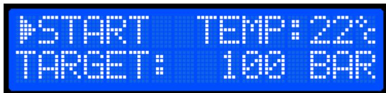
With the start display visible, press the rotary control knob once to start the compressor. After starting the compressor, the running display will appear.
